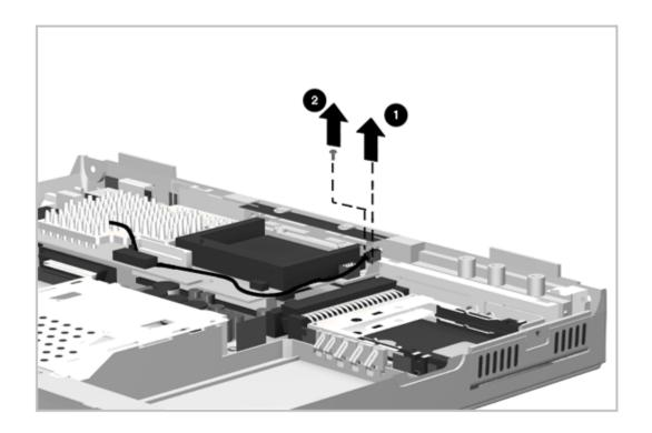
Figure 5-50. Removing the Processor Board Cable and Screws
